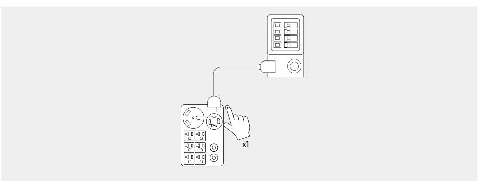
2. Double-press the AC outlet button to turn on EV mode, wait until the car icon appears on screen, then connect your device to the L14-30R AC output port. When the power station is in EV Charging mode, it cannot be charged via AC simultaneously.
