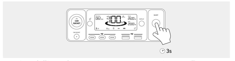
Press the On/Off button for 3 seconds to turn your power station on or off. When the "Remaining Battery" indicator shows on the LCD screen, your power station is ready to charge devices.
