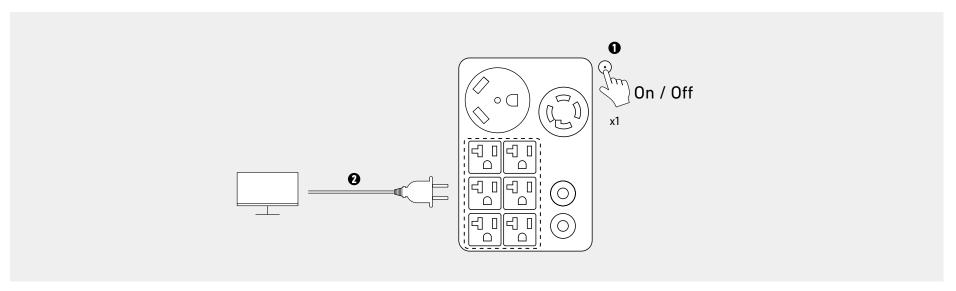
Press the AC outlet button and connect your devices to the TT-30R AC output ports. The max output power via this port is 3000W.
