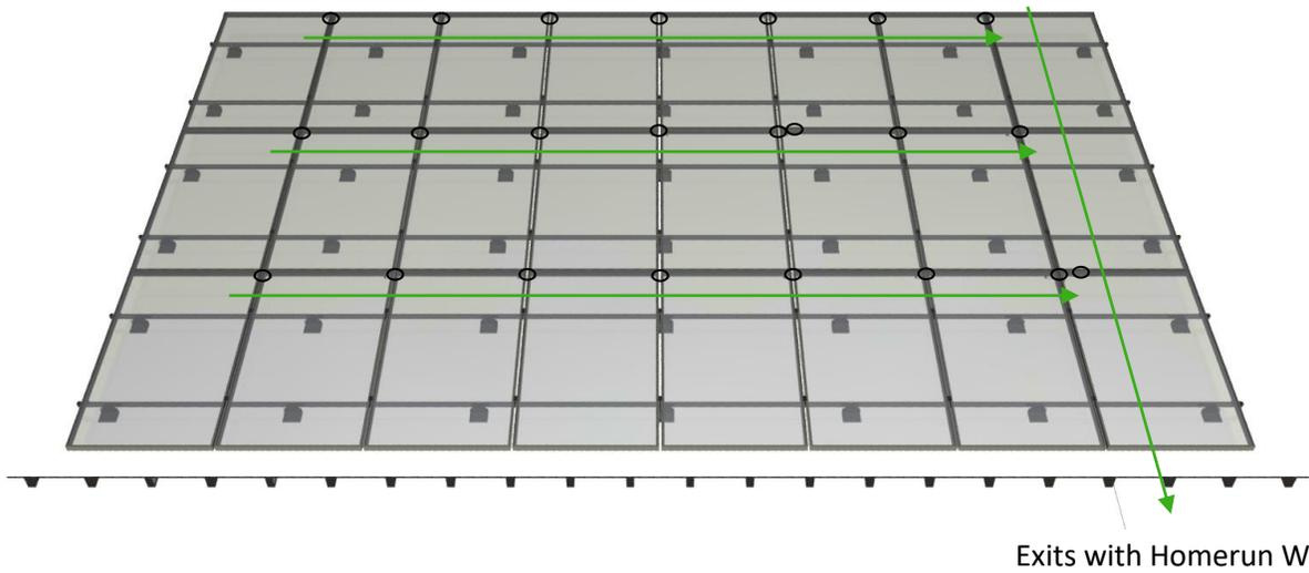
Step 2: Locate the DynoBond between your first set of modules. The DynoBond penetrates the anodization of the module's frames; bonding them together. The DynoBond is used as a jumper between modules acting as a bridge for the equipment ground path. The connection points can be made along either the short or long sides of the panels granted the frame is the same on all four sides of the module.
