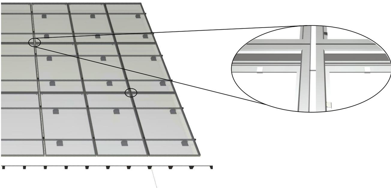
Step 6: The homerun equipment ground wire can be landed via a grounding lug attached to a grounding point of a module anywhere throughout the array. Please keep in mind if a panel is removed within the array at any point for maintenance or service a DynoBond should be placed to maintain ground continuity. This replacement DynoBond is highlighted in red for clarity.
