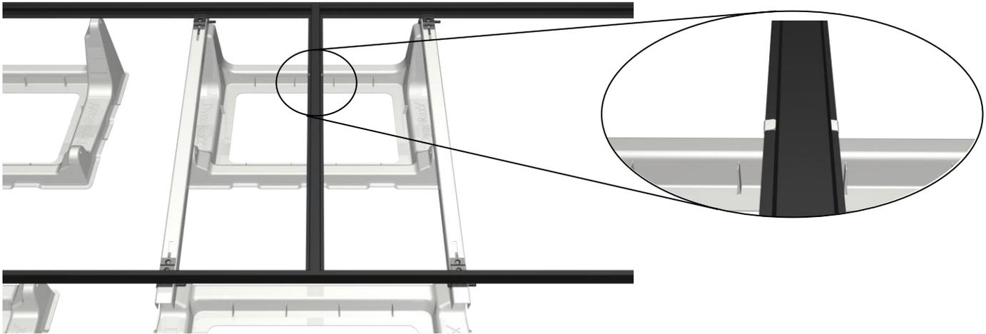
Step 3: Position the DynoBond on the bottom lip flange of the first module. To engage the module frame fit the module's bottom lip flange between the toothed section of the stainless-steel spring clamp. Next, fit the adjacent module with the remaining free end of the DynoBond. Place a bend or an "S-curve" in the conductor to allow for thermal expansion and contraction of modules within an array.
