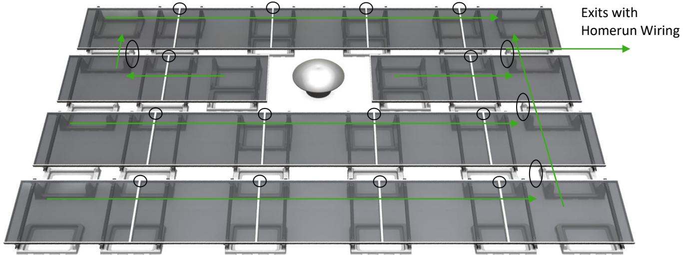
Step 2: Locate the DynoBond between your first set of modules. The DynoBond penetrates the anodization of the module's frames; bonding them together. The DynoBond is used as a jumper between modules acting as a bridge for the equipment ground path. The connection points can be made along either the short or long sides of the panels granted the frame is the same on all four sides of the module.
