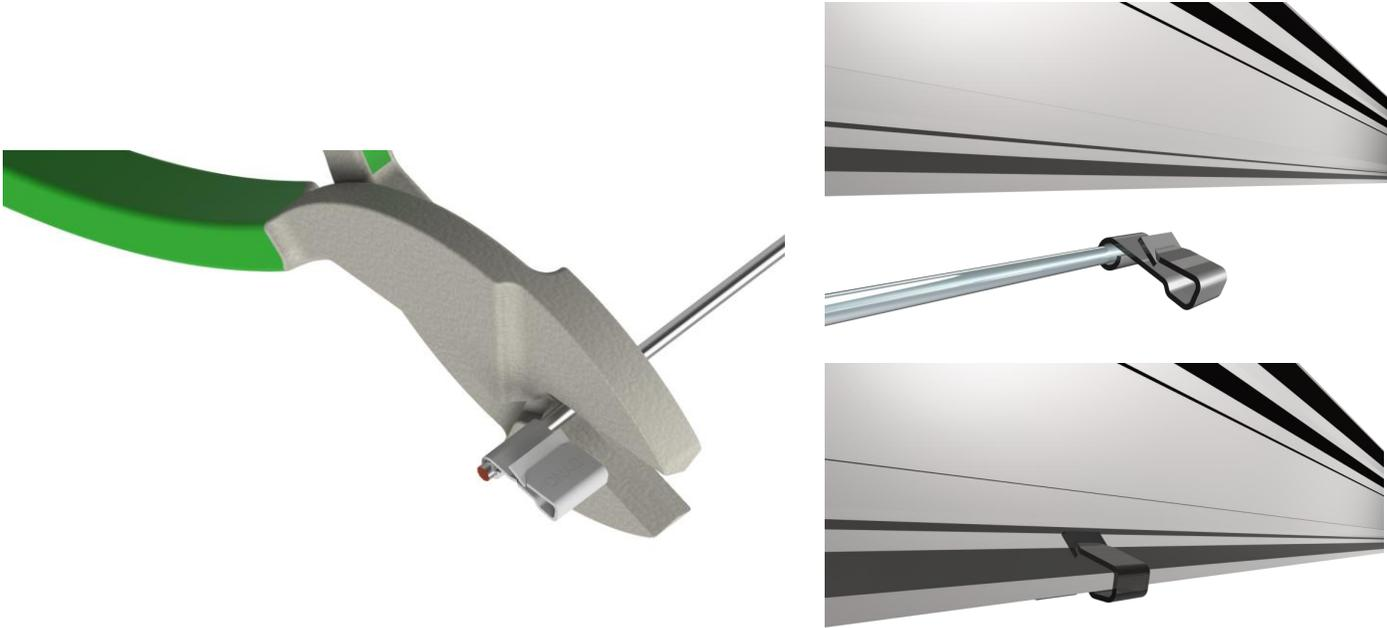
Step 2: Route tin-plated copper to termination or splice point. If exiting a protected area of the area take extra precautions to protect tin-plated copper wire in conduit. In below example, the DynoBond is being terminated within a junction box.
