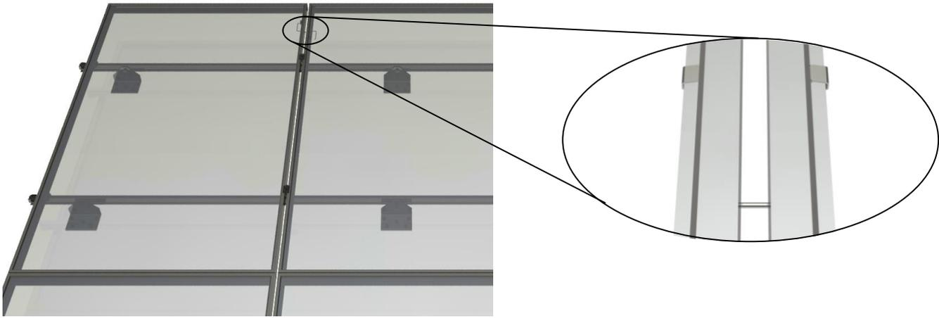
Step 3: Position the DynoBond on the bottom lip flange of the first module. To engage the module frame fit the module's bottom lip flange between the toothed section of the stainless-steel spring clamp. Next, fit the adjacent module with the free end of the DynoBond. Place a bend or an "S-curve" in the conductor to allow for thermal expansion and contraction of modules within an array.
