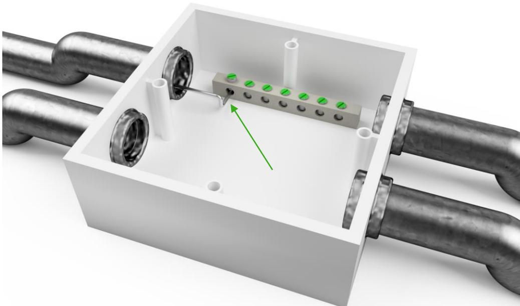
Step 3: Terminate or splice equipment ground. In the below example, equipment ground is terminated within a junction box.
