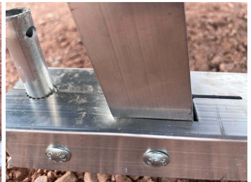
PHOTO 15: Upright deformation after testing
