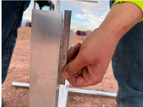
PHOTO 10: Slight deformation after load removed
