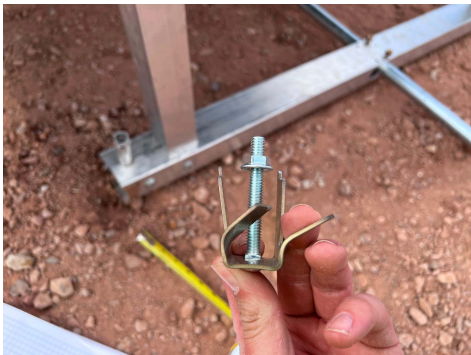
PHOTO 13: Bracket deformation after testing
