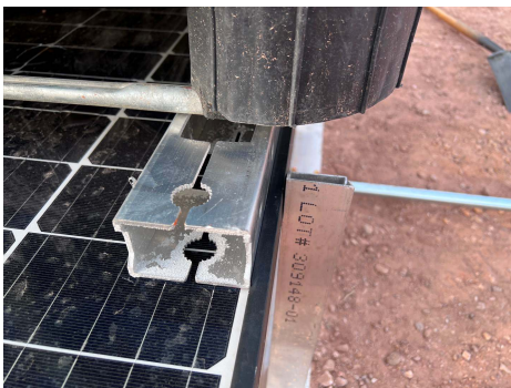
PHOTO 7: Slight deflections noted under load
