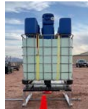
PHOTO 6: Slight deflection under load
