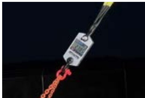
PHOTO 8: Closeup of max load, 2385 lbf
