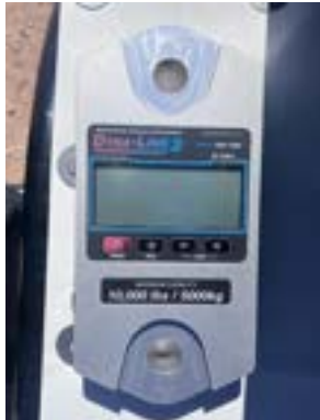
PHOTO 1: Dynamometer used to record loads
