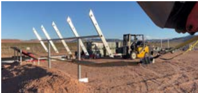
PHOTO 1: Horizontal force test setup
