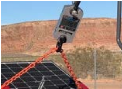
PHOTO 10: Test 2 - Load at ballast shift
