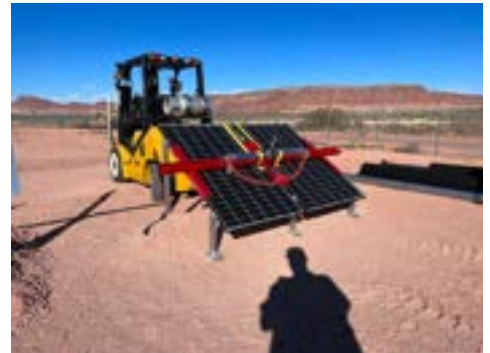
PHOTO 3: Test setup - IR-30 Solar Racking System with red test cross frame
