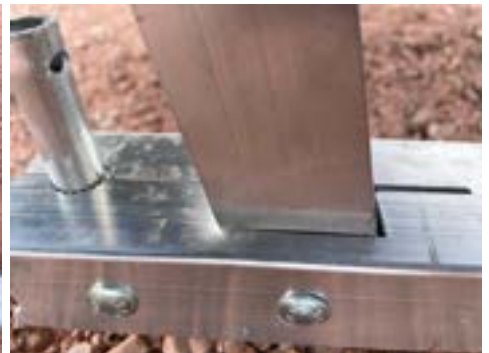
PHOTO 15: Upright deformation after testing
