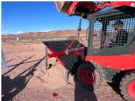
PHOTO 4: Test setup with dynamometer and chains connected
