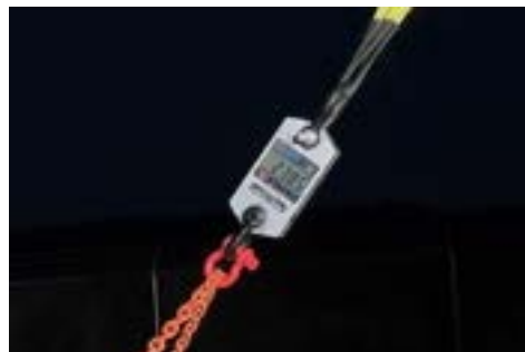
PHOTO 8: Closeup of max load, 2385 lbf
