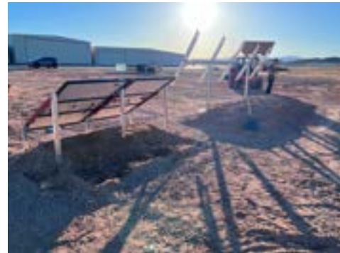
PHOTO 2: Horizontal force test setup
