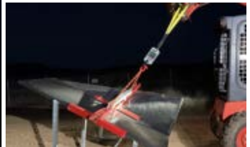
PHOTO 9: IR-30 Solar Racking System right after max load when panel failed
