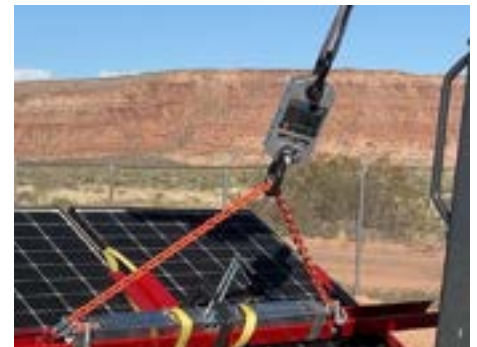
PHOTO 6: Test 1 - Load at ballast shift
