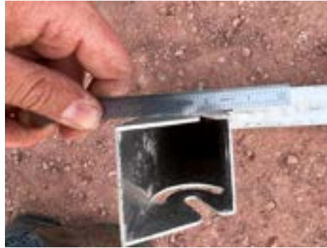
PHOTO 11: Slight deformation after load removed
