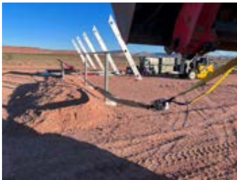
PHOTO 3: Horizontal force test setup
