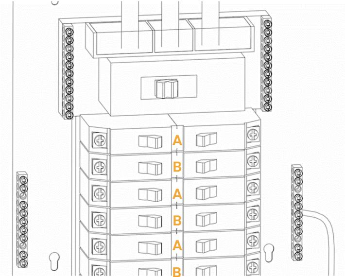
**NOTE:** For purposes of Lumin installation, the top row of breakers will *always* be classified as “A”. The second row of standard breakers will be “B”. The alternating A-B-A-B pattern continues down the rows of breakers. **Exception:** All breaker rows are designated “A” in panels with two-wire single-phase power rather than three-wire single-phase (split phase).
