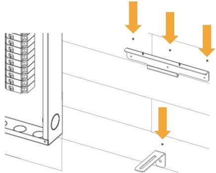
Marking Hole Locations Using Brackets
