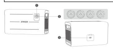
On/Off Button Long-press for 2 seconds to turn the expansion battery on and off.
