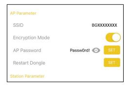
7. Select "SET" to save the password which will also enable WPA2 security. There may be a short pause after selecting the SET button. Press "OK" to verify the setup is complete. The dongle will reboot and should be back online within a couple minutes.
