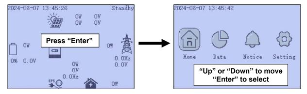
Press the "Down" arrow to move right, then press "Enter" to select. Once an item from the main menu is selected, use the following for navigation:
