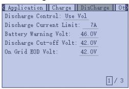
**Discharge Current Limit:** The discharge current limit is at 250A to support a single inverter. When running in parallel mode, set the max discharge to support the max current draw as a total from all connected inverters. If this setting is not adjusted and the inverter uses current greater than the default setting, the inverter will either shutdown or switchover to grid supplying the loads. Once the load returns to within specified settings, the inverter will switchover back to battery.
