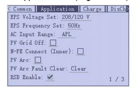
**EPS Voltage Set:** Verify the voltage is set to 240VAC.
