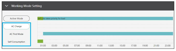
The "Working Mode" feature has several different preset working modes that allow the user to configure the system to meet their needs through customizing settings. Working modes for the EG4® 12000XP include AC Charge, AC First Mode, and Self Consumption.
