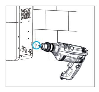
7. Remove the angle bracket and drill a hole at the marking. Use the drill bit size based on the anchor type or screw size as directed in step 3 (Repeat this step for both sides).
