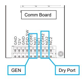
Dry Port Relay Maximum Specification: 250VAC 5A Gen Port Relay Maximum Specification: 250VAC 5A NO---Normal Open
