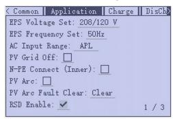
EPS Voltage Set: Verify the voltage is set to 240Vac
