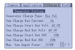
Using the EG4® Monitor Center, go to the "Maintenance" tab where "Remote Set" will be selected by default. Scroll to the "Generator Charge" section and select the "Generator Charge Type." Normally, lead-acid batteries are charged according to voltage and lithium batteries are charged according to SOC. For more information on the EG4 Monitor Center and generator settings, see section 12.
