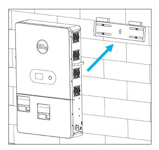
5. Using the team-lift technique, place the inverter on to the wall bracket securing it to the wall.
