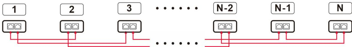
**Note:**  $N_{max}=12$ units Best practice is to minimize the number of jumps between inverters by alternating between 1 and 2 jumps on each inverter.
