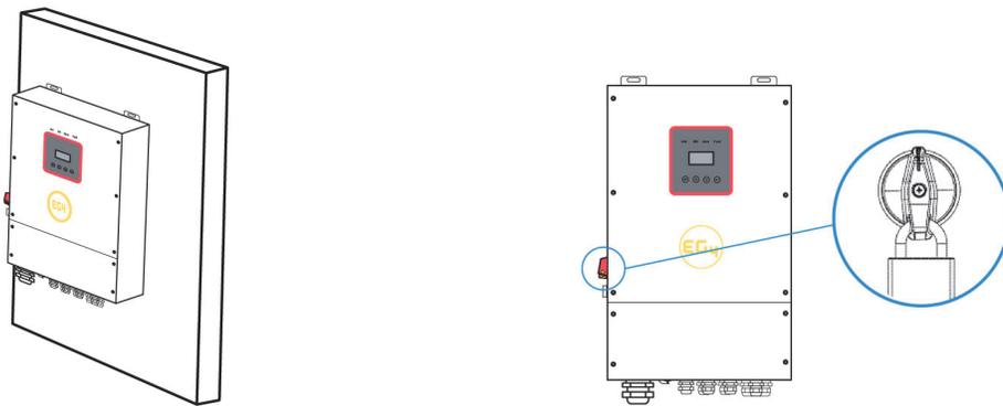
**Step 4:** Use an allen wrench to remove the cover screws, and remove the cover. Remove the waterproof cover with a flat-head screwdriver. Wiring box conduit plugs are provided for 1 inch conduit fittings. If conduit being used is not 1 inch, an appropriate conduit adapter should be used.
