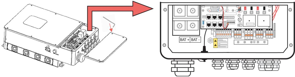
**Step 5:** Insert the conduit and fasten the joint.
