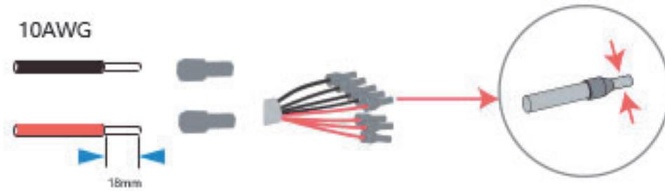
**Step2.** Feed the PV cables through the PV port, and connect the PV cables to the PV terminals.
