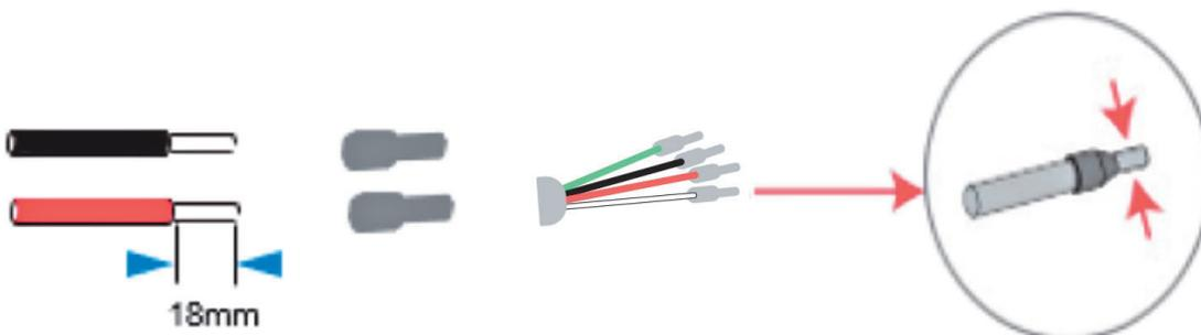
**Step4.** Feed the grid cables through the grid port and connect grid cables to grid terminals.
