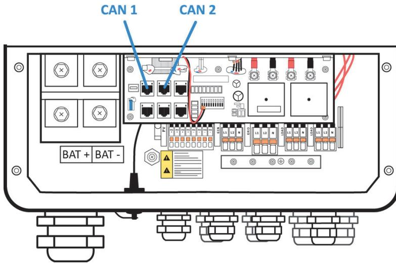
For parallel communication, CAT 5 cables are needed. When using common batteries, BMS cable needs to be connected to the master unit. The inverter shares the BMS information by inter-unit parallel communication cable.
