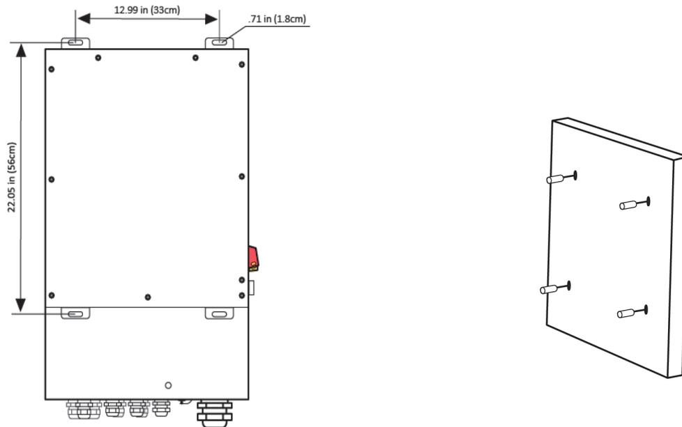
**Step 2:** Lift up the inverter and align the holes of the inverter with the expansion bolt, mount the inverter on the wall.
