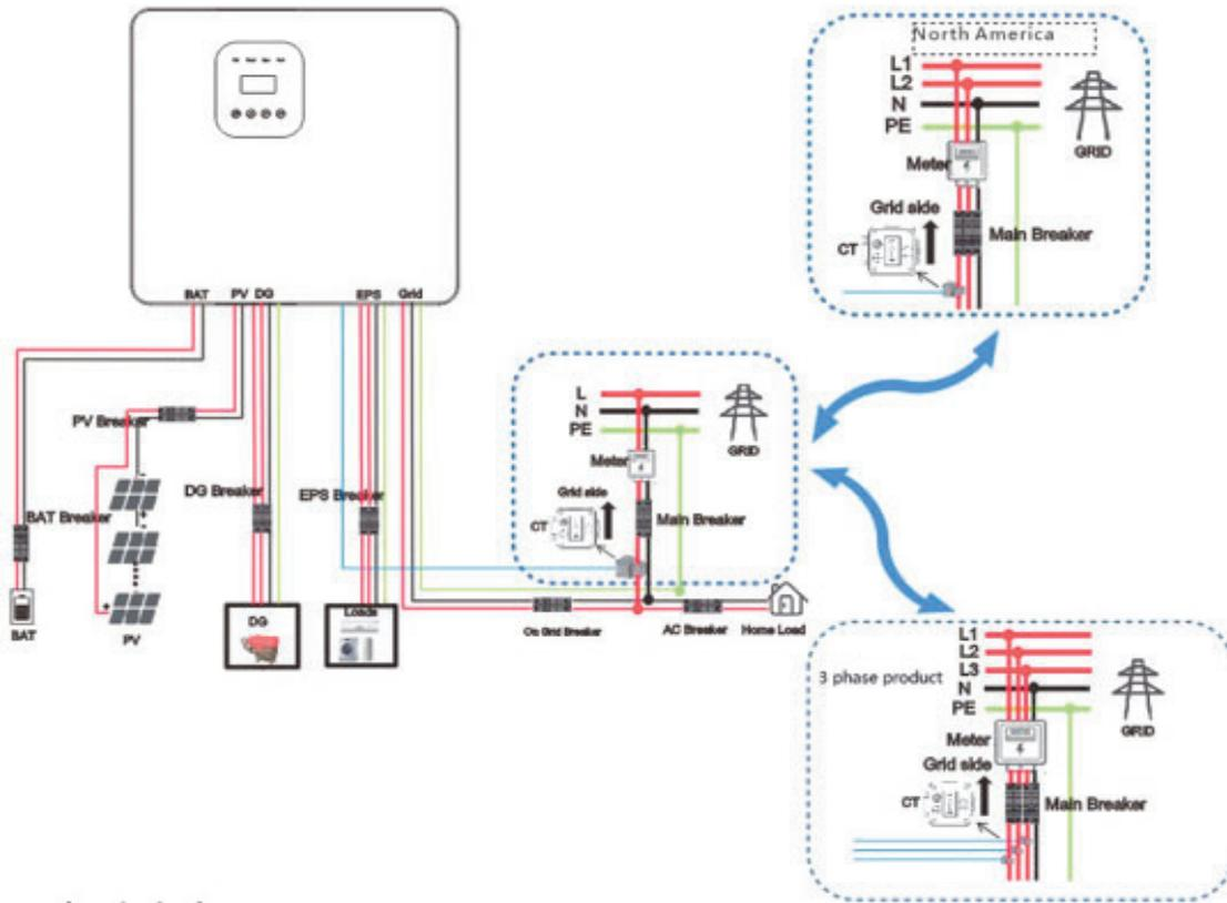
**Note:** The current transformers should be installed as shown in the figure above. Note that the CT crosses the L line, the CT arrow marks point to power GRID, RJ45 is connected to "Grid Current" in COM. If it is 3 phase products, will be 3pcs CT crosses to "L1, L2, L3" line.
