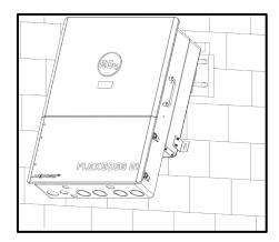
Temporarily mount the L-bracket to the side of the inverter (located at the bottom, one on each side). Mark holes on the wall based on the hole location on the Lbracket (repeat this step for both sides).
