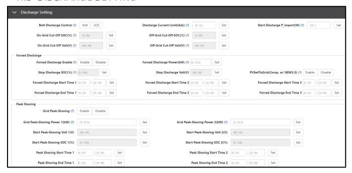
Batt Discharge Control: If the inverter communicates with the lithium battery and is capable
