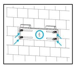
5. Using the team lift technique, place the inverter onto the wall bracket, securing it to the wall.
