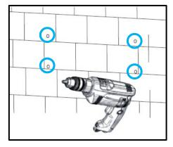
4. For concrete or brick installation, insert the expansion bolts into the drilled holes. Install the bracket to the wall, ensuring the arrow is pointing up. Use the corresponding nuts and washers (packaged together with the expansion bolts) to affix the bracket to the wall. For stud wall installation, use the proper screws and affix the bracket to the wall.
