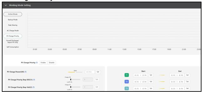
The order of priority for solar power usage will be Battery >Load >Grid. During the "PV Charge Priority" period, loads are first supplied power from the grid. If there is excess solar power after charging batteries, the excess solar will power the loads along with grid power.
