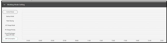
The station will default to Self Consumption mode. The order of priority for powering loads is Solar > Battery > Grid. The order priority for solar power is Load > Battery > Grid which creates an ideal scenario when needing to prioritize solar power generation over other types of power. Self Consumption mode will increase the self-consumption rate of solar power and reduce energy bills significantly. Effective when Charge Priority, AC Charge, and Forced Discharge are disabled.
