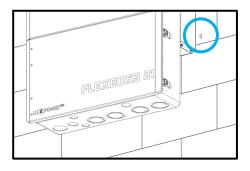
8. Attach the L-brackets (one on each side) to the inverter and to the wall using the correct hardware. Once the bracket is secure, the wall installation is complete.
