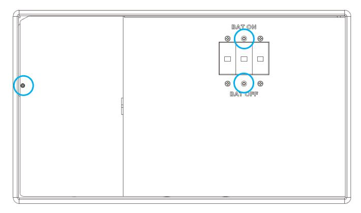
Once the cover is open, follow the sections below for connecting the wiring for PV, battery, AC, parallelled inverters, and rapid shutdown. Before connecting any wiring to the inverter, verify each wire is not carrying voltage using a multimeter.
