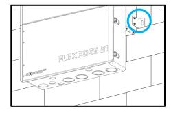
7. Remove the L-bracket and drill a hole at the marking. Use the drill bit size based on the anchor type or screw size as directed in step 3 (repeat this step for both sides).
