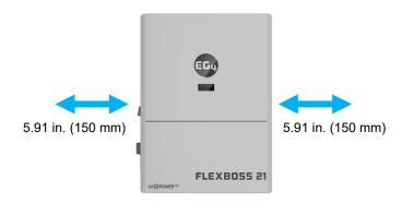
3. Never position the inverter in direct sunlight, rain, or snow. Refer to the figure below and choose a well-shaded site or in an indoor location to protect the inverter from the elements. The inverter should be installed upright on a vertical surface.
