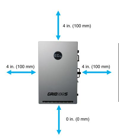
Be sure to maintain the spacing requirements shown in the image to allow access to fully open the door and to view the dongle LEDs.
