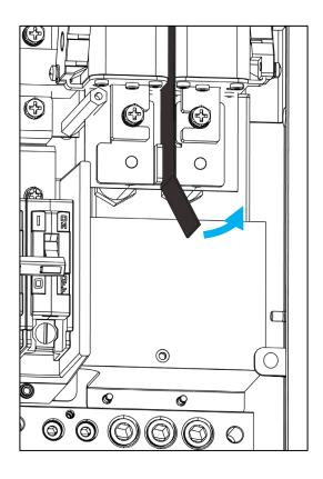
4. Install the Eaton (model (CSR2200N) CSR25K) breaker by sliding it into place, aligning the bolt holes in the breaker lugs to the holes on the busbar.
