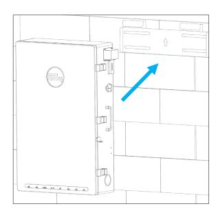
5. Using the team-lift technique, place the GridBOSS onto the wall bracket securing it to the wall.
