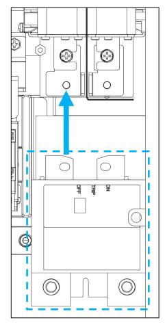
5. Using a 10 mm socket, install the two M6 screws in the busbar, then install the M4 screw that holds the opposite end of the breaker in place.
