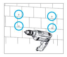
3. When installing the bracket to <u>concrete or brick</u>, drill 25/64-inch (10 mm) diameter holes on the marks, making sure the holes are deeper than 3-3/16 in. (80 mm) when using the included expansion bolts.
