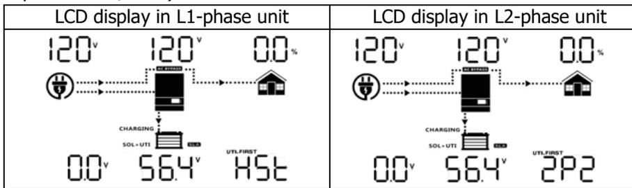
Step 5: If there is no more fault alarm, the system with split phase output is completely installed.
