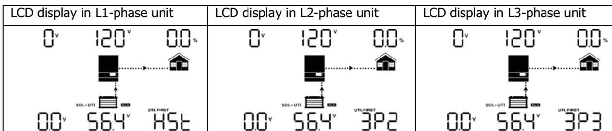
Step 4: Switch on all AC breakers of Line wires in AC input. If AC connection is detected and three phases are matched with unit setting, they will work normally. Otherwise, they will display warning 15/16 and will not work in the line mode.
