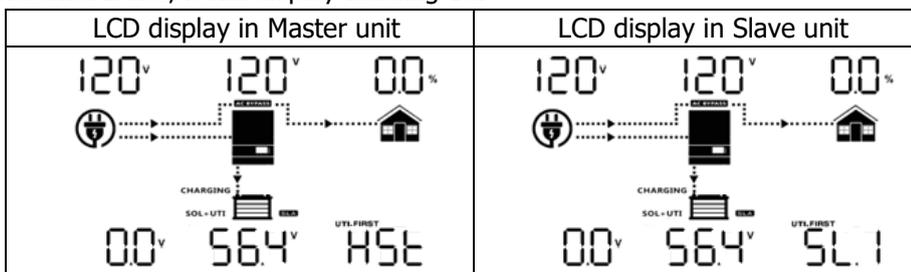
Step 5: If there is no more fault alarm, the parallel system is completely installed.
