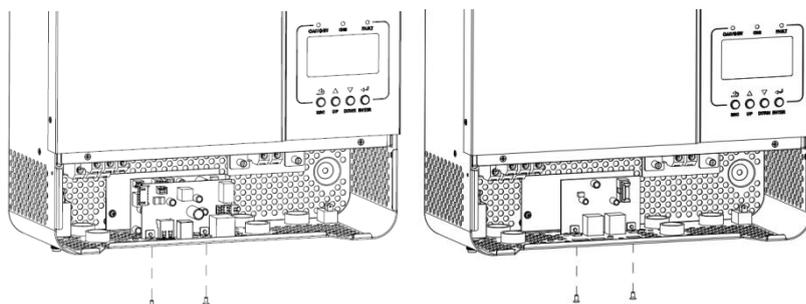
**Step 3:** Remove two screws as below chart and remove 2-pin and 14-pin cables. Take out the board under the communication boards.
