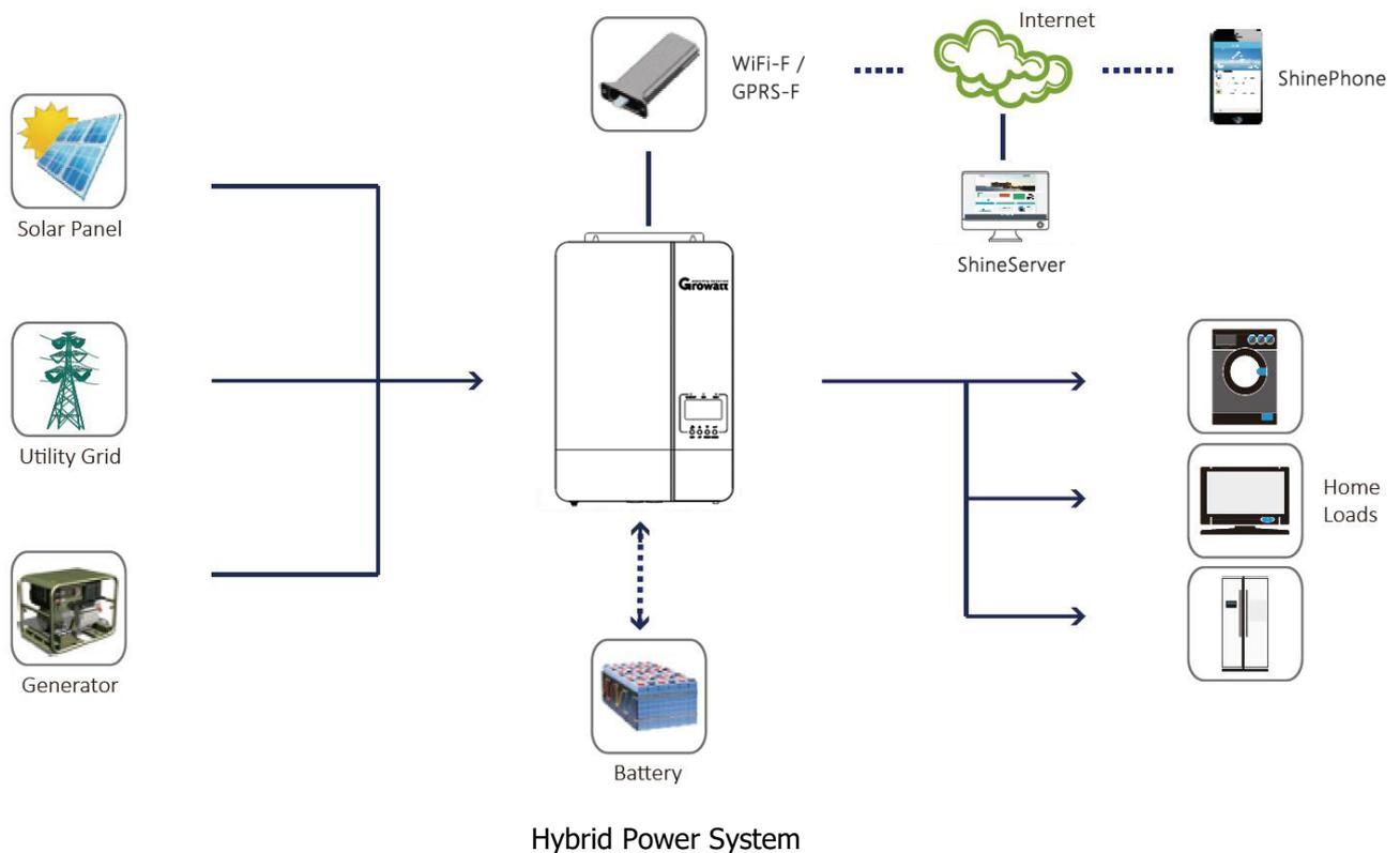
This is a multifunctional off grid solar inverter, integrated with a MPPT solar charge controller, a high frequency pure sine wave inverter and a UPS function module in one machine, which is perfect for off grid backup power and self-consumption applications. This inverter can work with or without batteries.
