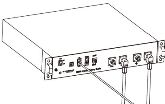
**Note:** If choosing lithium battery, make sure to connect the BMS communication cable between the battery and the inverter. You need to choose battery type as "lithium battery".
