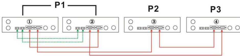
Two inverters in two phases and only one inverter for the remaining phase:
