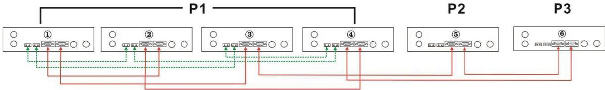
**WARNING:** Do not connect the current sharing cable between the inverters which are in different phases. Otherwise, it may damage the inverters.
