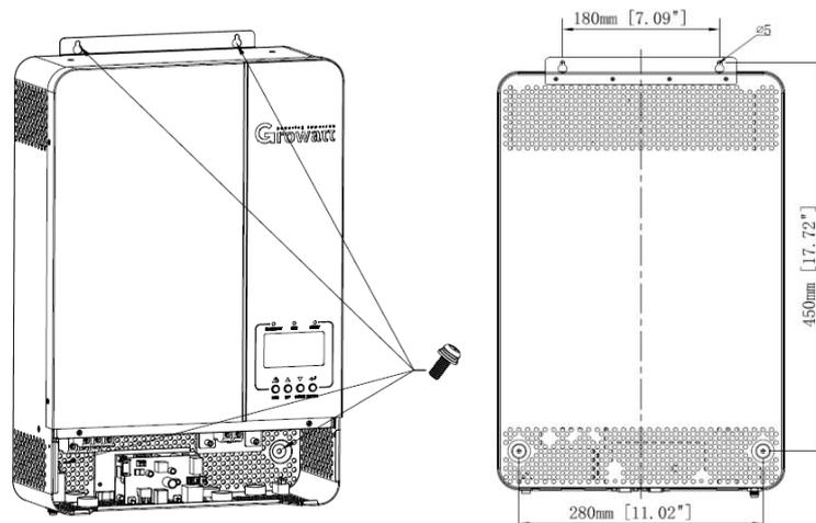
Install the unit by screwing three screws. It's recommended to use M4 or M5 screws.
