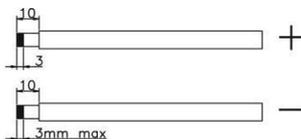
2. Check correct polarity of connection cable from PV modules and PV input connectors. Then, connect positive pole (+) of connection cable to positive pole (+) of PV input connector. Connect negative pole (-) of connection cable to negative pole (-) of PV input connector.
