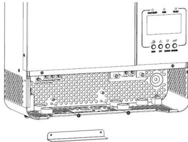
**Step 5:** Install new parallel board with 2 screws tightly.
