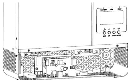
**Step 8:** Put wire cover back to the unit. Now the inverter is providing parallel operation function.
