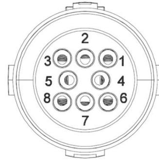
Insert the stripped and bared cable through pressure screw, sealing, threaded sleeve in sequence, insert cables into connection terminal according to number indicates on it and tighten the screws firmly .Please try to pull out the wire to make sure the- it is well connected.
