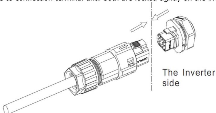
Press the fasteners and pull it out from the inverter.
