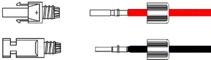
Tighten the nuts to finish the wiring.
