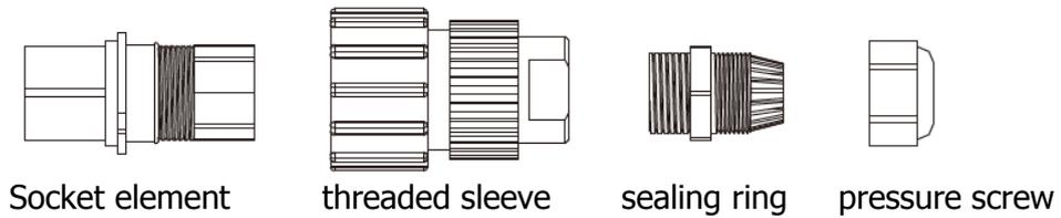
Insert the stripped and bared conductors U, V, W, PE in to screw terminals with sign U, V, W, PE on the socket element and tighten the screws.
