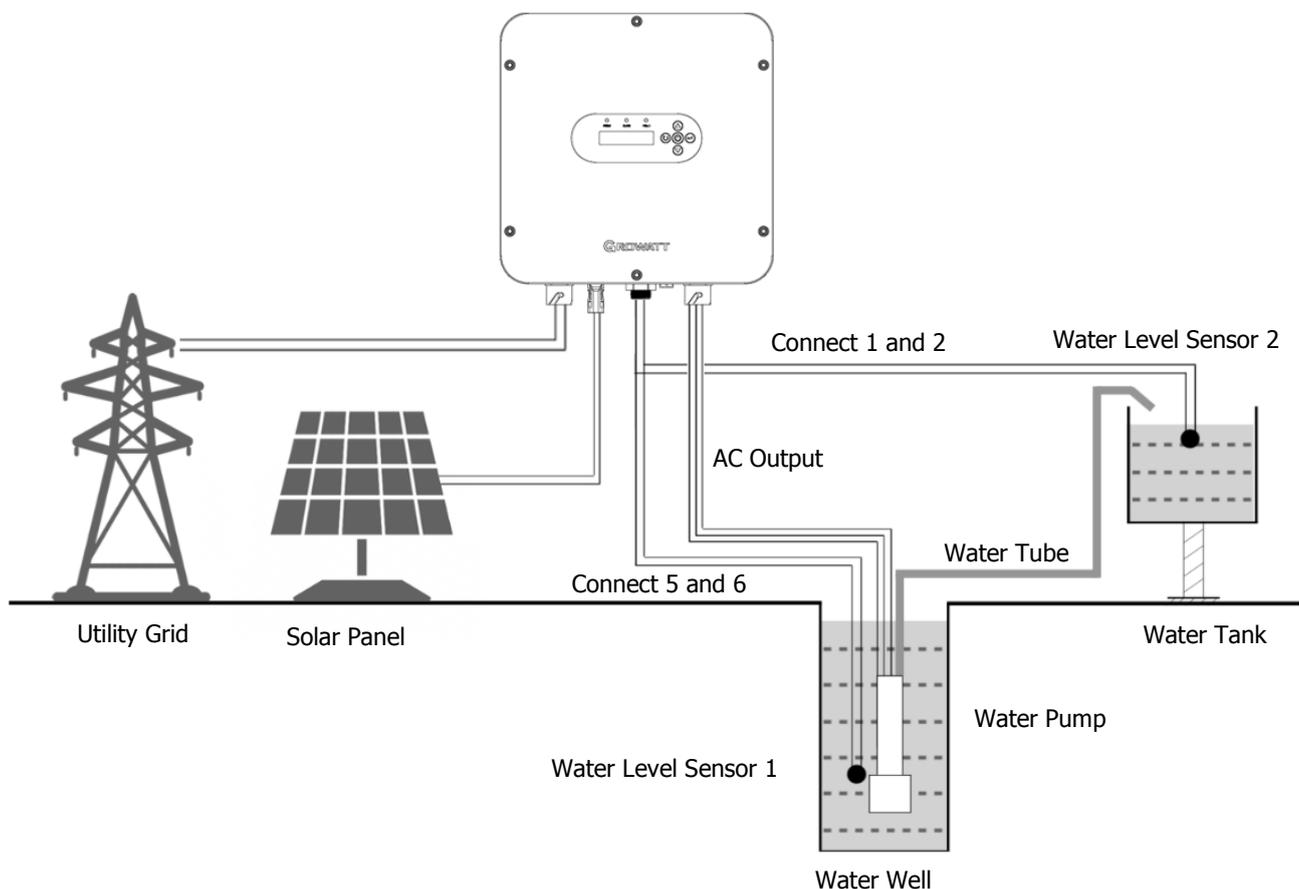
**!** Notice: connect water level sensor 1 and detect water shortage. Respectively connect two signal lines of sensor with 5 and 6 of COM terminal. When water level sensor 1 detects that the water level of well is lower than the level set by sensor, the pump inverter will delay for 5s, then turn off output protection pump. The water level recovers. Wait for 20s, then the pump inverter re-works normally.
