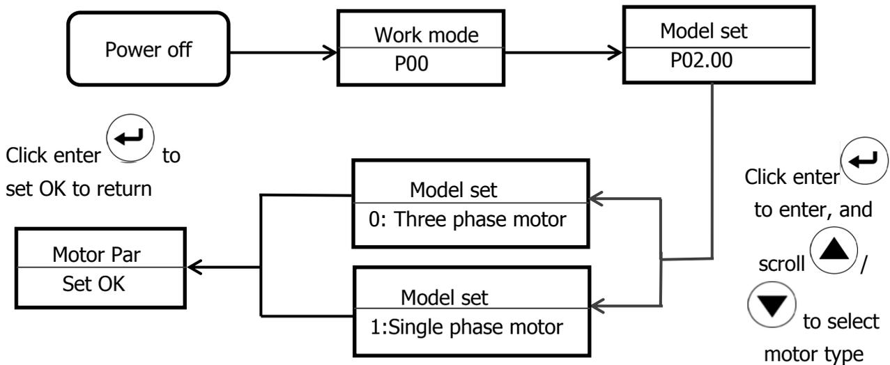
When the three-phase motor is set to the single-phase motor, the P02.05 needs to be changed to the corresponding single-phase motor current.
