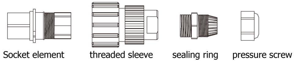
Insert the stripped and bared conductors L, N, PE in to screw terminals with sign L, N, PE on the socket element and tighten the screws.
