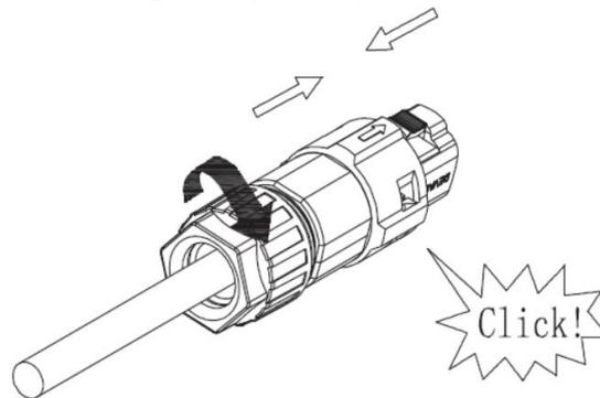
Push the threaded sleeve to connection terminal until both are locked tightly on the inverter
