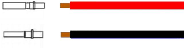
Crimp contact barrel by using a hex crimping die. Put the contact barrel with striped cable in the corresponding crimping notch and crimp the contact. Insert the core tube into slot of connection until hear the sound indicating fit in place.
