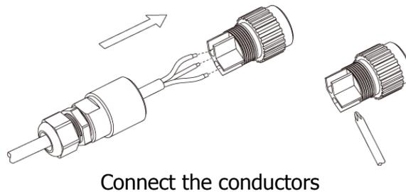
Push the threaded sleeve in to the socket element. Screw the pressure screw tightly onto the threaded sleeve.
