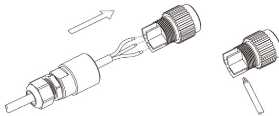
Push the threaded sleeve in to the socket element. Screw the pressures crew tightly onto the threaded sleeve.
