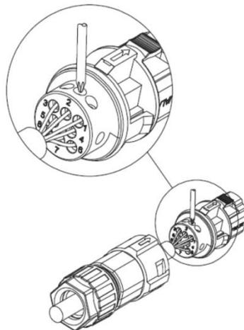
Push the threaded sleeve into the socket .Tighten up the cap on the terminal.
