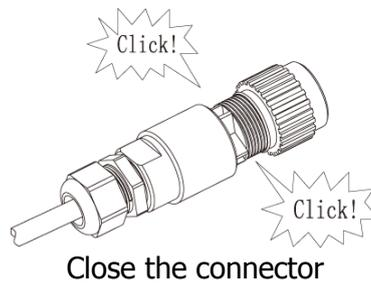
Insert the AC connection plug into the AC connection receptible on the inverter.
