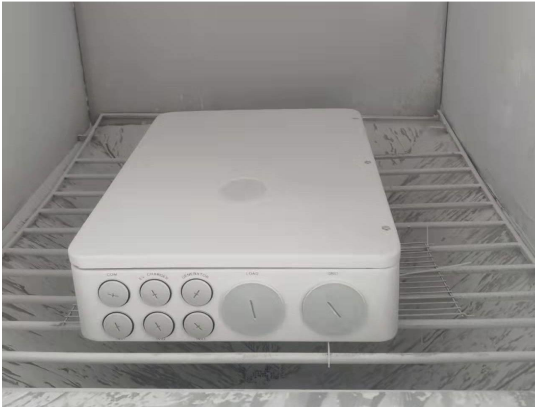
Test setup of IP6X
