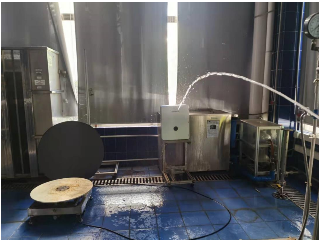
Test setup of IPX5
