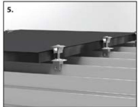
**6. Install Additional PV Modules-repeating steps 3-5:** place another module in the MidGrabs that were left open in the previous step. Tighten the downslope row of grabs each time a module is placed and leave the upslope open until the next module is placed (Fig. 6). The final row will be finished with EdgeGrab/StandOff Assemblies. Periodically look back at the modules you've installed to double check that the MidGrabs were tightened.
