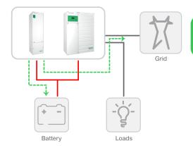
Just like Smart Charge for AC Coupled systems, Enhanced Grid Support is designed to maximize and prioritize storage loads. The value of this feature is that the stored energy can be used later when rates are higher (Time-of-Use). Or in applications where the grid is intermittent, EGS prioritizes storage of your PV production to maximize readiness for potential grid outage.
