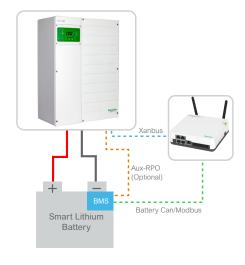
Lithium-ion battery with closed loop control
