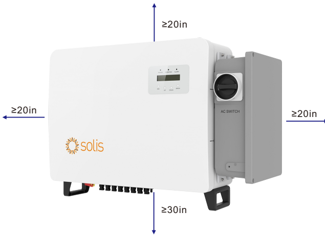
Figure 3.2 Clearance distances requirement for the inverter
