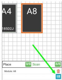
7. To manually enter TS4 data, tap the module in the layout grid, tap the blue barcode icon, and enter the code.
