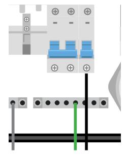
To connect the ATS to generator power output, connect four 4 - 1/0 AWG conductors to the ATS generator neutral and ground busbars and L1/L2 terminals.
