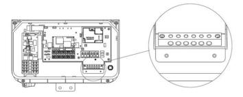
Grounding electrode conductor (GEC):
