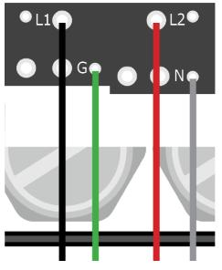
2. Terminate conductors at a main or essential loads panel.
