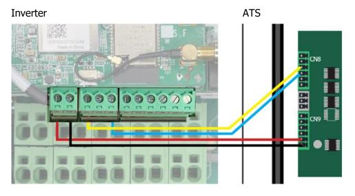
To connect to the inverter *GRID* terminals:
