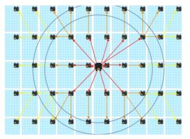
The TAP communicates directly with any TS4 within 10 m (33 ft.). Each TS4 can relay data to and from another TS4 within 10 m (33 ft.). The TAP can communicate through relays to any TS4s within 35 m (115 ft.).
