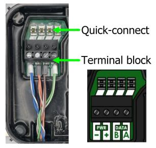
3. At the inverter, terminate the wires at the 4-pin TAP plug from bottom to top: –, +, Data B, Data A.
