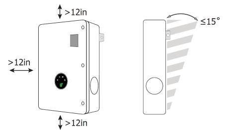
2. Use screws appropriate for the wall surface to affix the bracket, hang the ATS, and secure it with an M5 screw.
