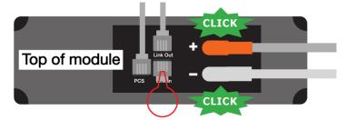
8. Insert an RJ45 terminator in the *Link In* terminal.
