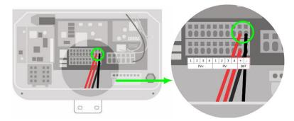
12. In the battery expansion wireboxes, connect a terminator to each CAN/COM terminal.
