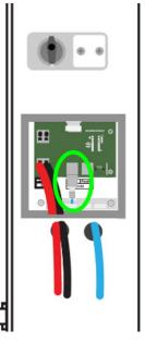
2. Plug the cable into the inverter battery COM port.
