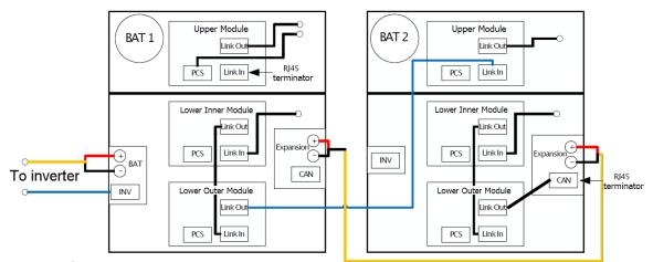
3. Insert a terminator in the battery #2 battery expansion wirebox CAN/COM terminal.
