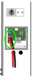
2. Connect the conductors to the inverter *BAT+* and *BAT-* terminals.
