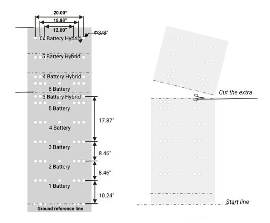
Cutting and placing the drill template
