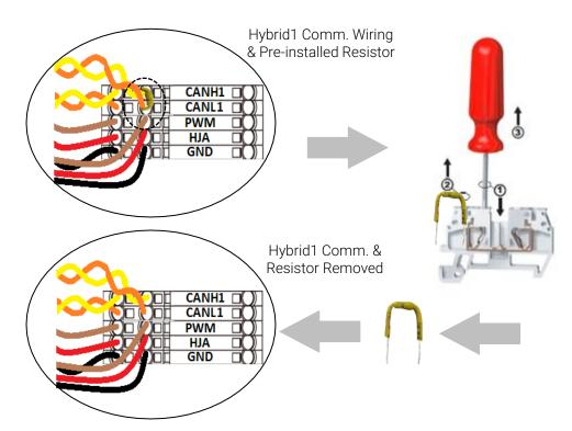
Note: The Final Hybrid (Hybrid2) unit that is last connected in the chain starting from the smart gateway communication terminals must need pre-installed resistor. Do not remove the resistor between the Comm terminals of the Final Hybrid (Hybrid2) unit.
