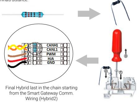
Step b. Push the spring terminals with the help of a flat head screw driver.
