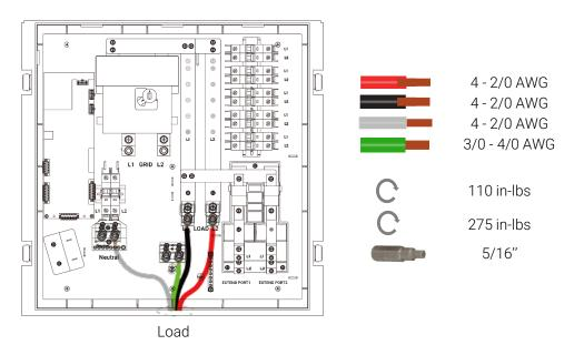
Figure 6. Smart Gateway Backup Load Wiring
