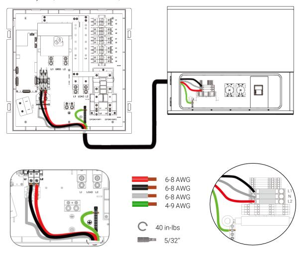
Figure 2. Smart Gateway to Hybrid AC Wiring
