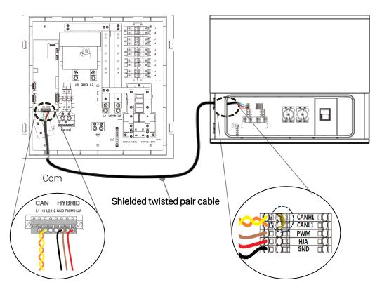
Figure 3. Smart Gateway to Hybrid Communication Wiring with Pre-installed Resistor
