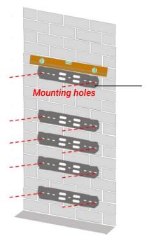
Install bracket C on wall
