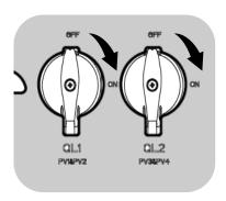
c. Turn on Hybrid-1 Circuit Breaker in the smart gateway.
