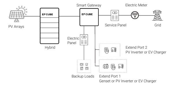
NOTE: The Smart Gateway is not rated to act as service entrance panel. If the utility meter doesn't have a circuit breaker (CB) or power panel between the Grid and Smart gateway, an MCB or power panel must be installed at the site.
