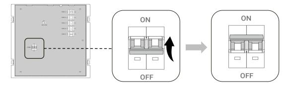
d. Turn on Smart Gateway Grid input power MCB in the electric panel.
