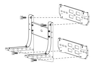
Fig. Attach bracket E and C
