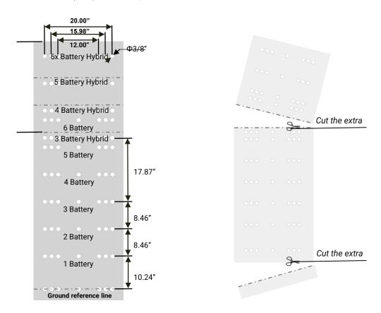
Cutting and placing the drill template
