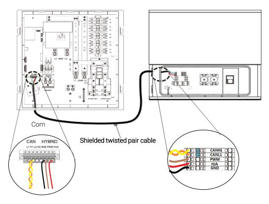
Figure 3. Smart Gateway to Hybrid Communication Wiring
