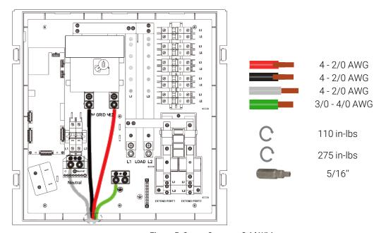
Figure 5. Smart Gateway Grid Wiring
