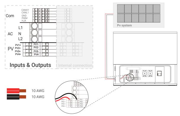
Figure 1. Hybrid to PV Array DC Input Wiring
