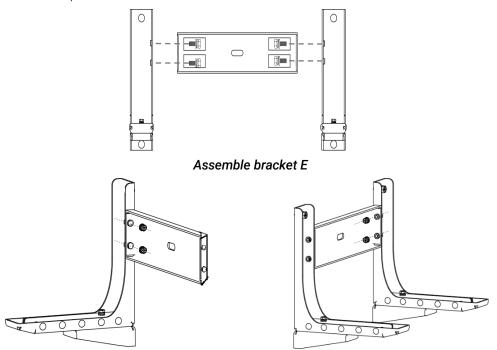
c. Attach the Bracket E to the Bracket C with bolts (M8\*0.79"), check that it is level using the level tool, and then tighten it with the socket wrench.
