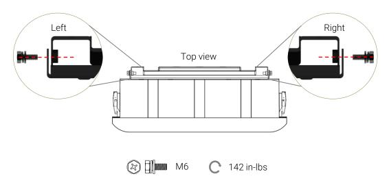
Tighten and check bracket A installations
