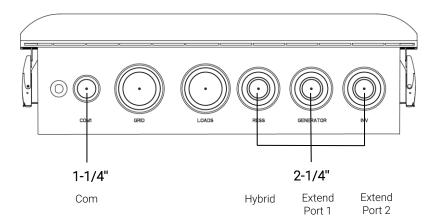
Figure 4. RESS and COM Knockouts
