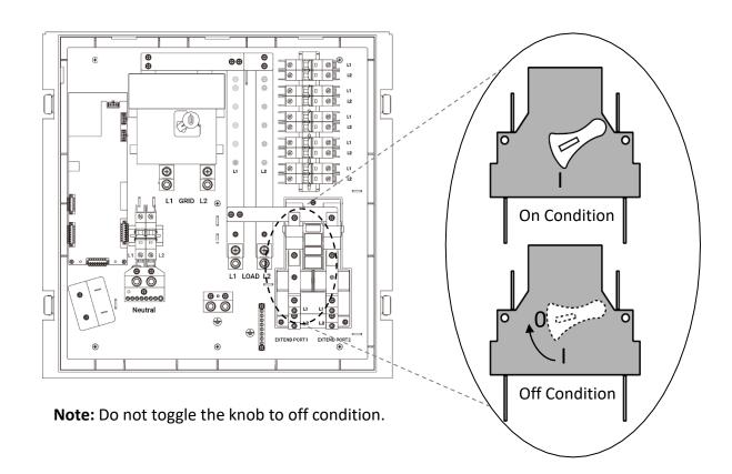
CAUTION: In accordance with the National Electrical Code (NEC), for Bus or Conductor Rating: The sum of the ampere ratings of overcurrent devices in circuits supplying power to a busbar or conductor shall not exceed 120% of the rating of the busbar or conductor". The installer must ensure that the Bus or conductors are not overloaded during the expansion of the EP Cube system.
