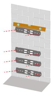
NOTE: Select the suitable M8 (or similar) bolt/screw to mount the Bracket C depending on the type of wall.
