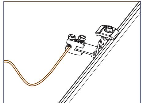
3) Each continuous array is connected to Equipment Grounding Conductor through Ground Lug (242-92202) installed on one module per array.
