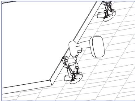
5) Lower the module to the roof and drive the (4) pre installed Snapnrack #14 Wood Screws with 1/2" hex head into the roof sheathing.
