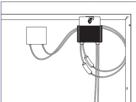
4) Connect the module leads to the input connectors on the MLPE device and manage conductors with the integrated Smart Clip.
