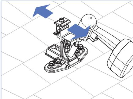
4) Loosen Course Adjustment bolt and adjust end Mounts up or down until aligned with bottom edge of array as marked on the roof, then tighten the Course Adjustment bolt.
