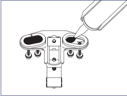
2) Fill both cavities on bottom of TopSpeed™ Mount created by SpeedSeal™ gasket with roof sealant to ensure a watertight seal.
