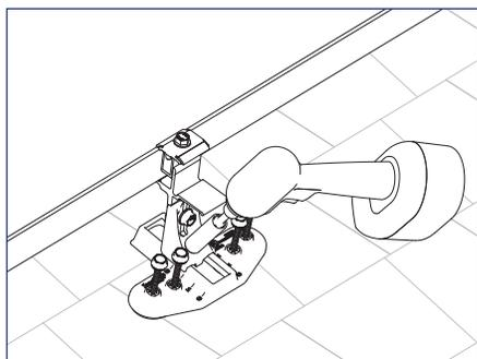
3) When module is level with roof verify the Speedseal™ portion of the TopSpeed™ Mounts are positioned entirely on one course of composition. If required listen the 1/2" nut and adjust the base as needed then tighten the bolt.
