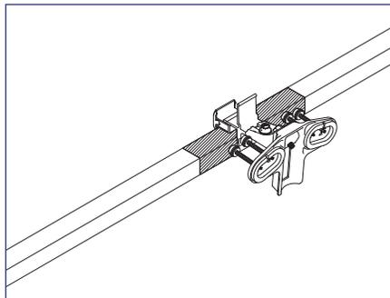
2) Position TopSpeed™ Mount clamp on the module frame within the module manufacturers required clamping zone.
