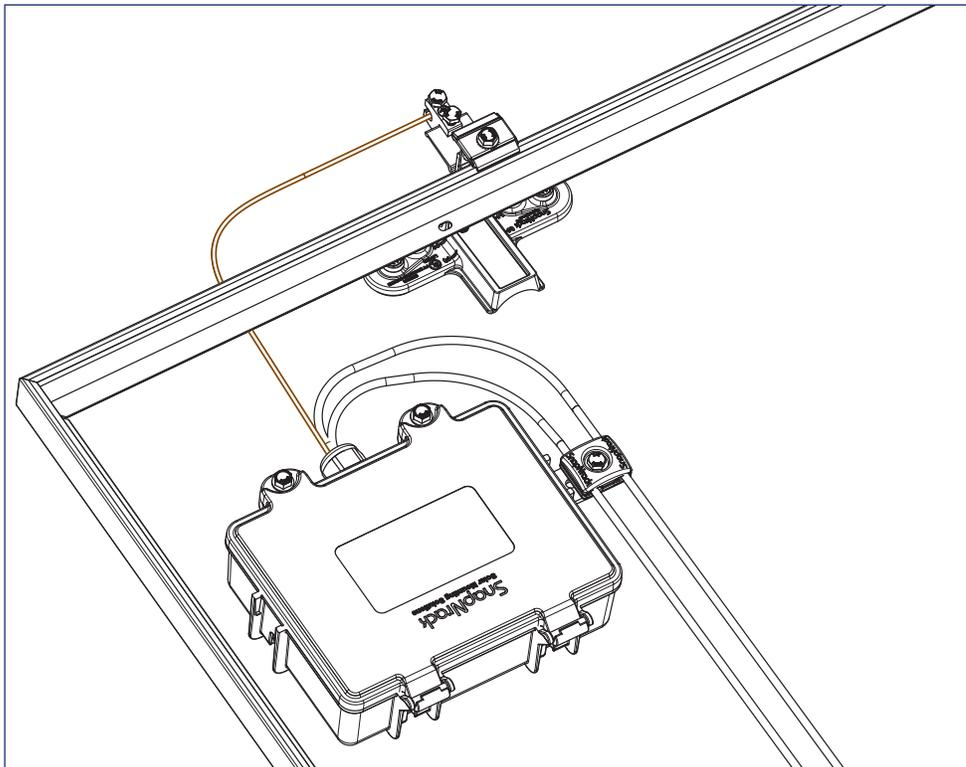
4) Optionally; Install Ground Lug on the Mount Landing Pad at the top of the array. Run bare copper between ground lug and Junction Box.
