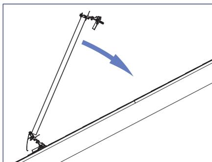
2) Lower upslope edge of module while simultaneously applying slight pressure to seat module into Mounts and/or Clamps.
