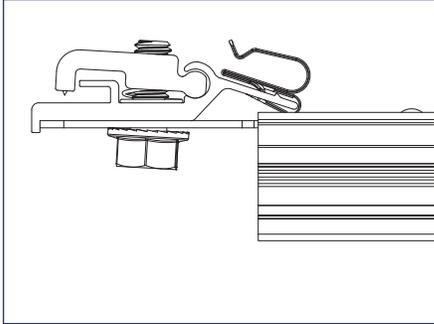
1) Slide the backplate channel of the MLPE device under the MLPE Frame Attachment Kit bolt. The MLPE mounting plate should rest against the MLPE mounting plate backstop on the MLPE Frame Attachment Kit.
