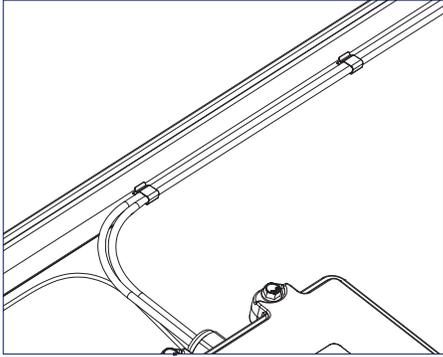
1) Use SnapNrack Smart Clip II to manage up to two PV wires inside the module frame while prepping out the modules on the ground or installing modules on the roof.
