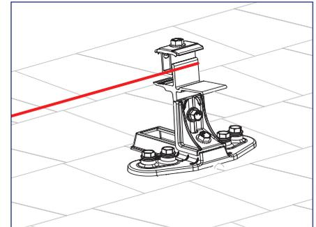
6) Pull string line tight from one corner mount to opposite corner mount to align and level all TopSpeed™ Mounts between the end mounts.
