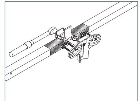
3) Tighten 1/2" clamping bolt to 16 ft-lb. Only two Mounts are required per module on one side.
