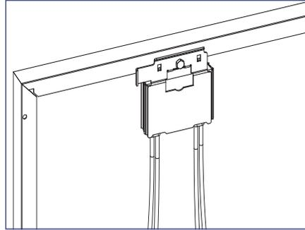
2) Install the optimizer mounting plate onto the module frame and tighten hardware to 11 ft-lbs.
