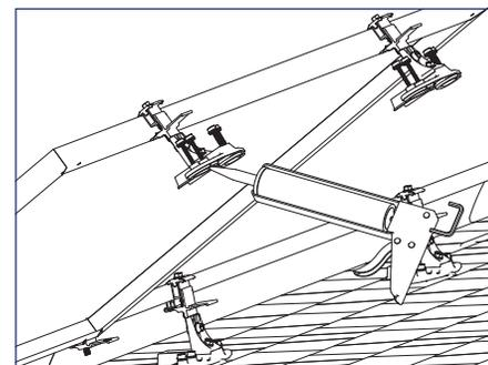
4) Lift the upslope edge of the module and fill the SpeedSeal™ reservoir with roofing sealant.
