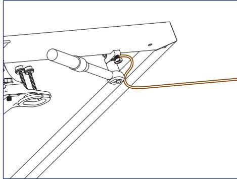
2) Run 10 - 6 AWG, solid, bare copper GEC into Ground Lug channel, torque wire clamping bolt to 8 ft-lb.
