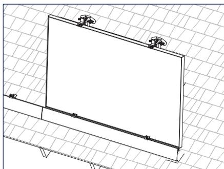
1) Rest downslope edge of module on the Mounts and/or Clamps position module so side edge is flush with marked edge of array layout or Skirt.
