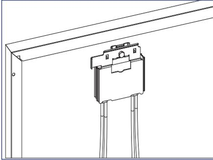
1) Locate the SolarEdge optimizer with Frame-Mounted Module Add-On at a location on the module frame that will not interfere with the TopSpeed™ Mounts.
