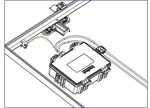
3) Run bare, solid EGC from Ground Lug R to Junction Box, bond bare EGC to stranded EGC in Junction Box. For details on installing the Junction Box reference the **Junction Box Installation Manual**.
