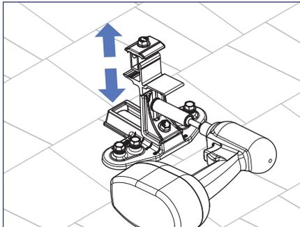
5) To set the TopSpeed™ Mount level loosen the Leveling bolt and move the clamp up or down, then tighten the Leveling bolt and torque to 16 ft-lb.
