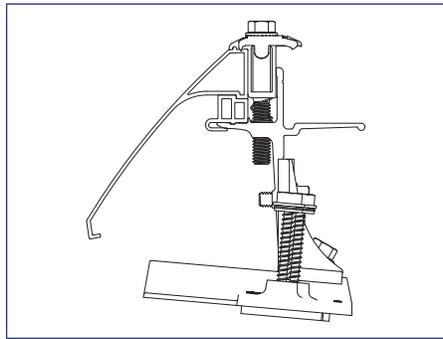
2) Column to column bonding provided by Universal Skirt and bonding clips in the Clamp assembly and/or the RL Universal Link assembly.
