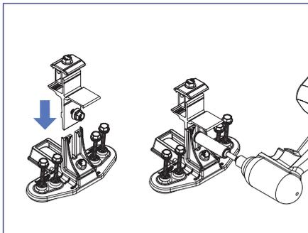
1) Assemble all TopSpeed™ Mounts required for the installation. Slide the clamp tower assembly into the angle bracket riser and tighten the leveling bolt to 16 ft-lbs.
