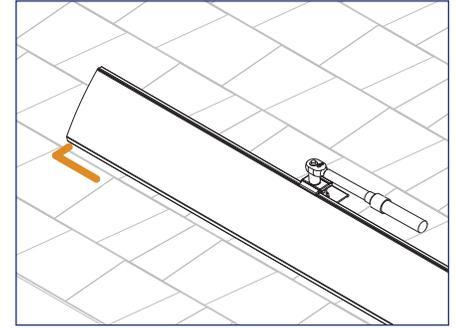
8) Install Universal Skirt by holding the skirt in Mount, sliding Skirt to align with array layout marks, and clamping skirt into mount.
