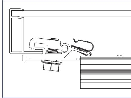
2) Position the MLPE Frame Attachment Kit on the module frame flange in a location that will not interfere with mounting system components. The module frame flange should rest against the module flange backstop on the MLPE Frame Attachment Kit.
