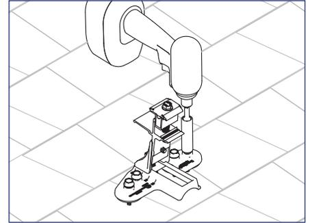
3) Attach TopSpeed™ Mount to roof using the (4) SnapNrack #14 Wood Screws with 1/2" hex head that are captured in the Mount.
