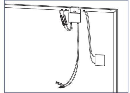
3) Connect the module leads to the input connectors on the optimizer and manage conductors with SnapNrack Smart Clips.
