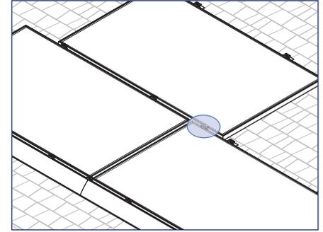
7) For staggered arrays and arrays with mixed orientation, use the TopSpeed™ Clamp as needed to support the modules.
