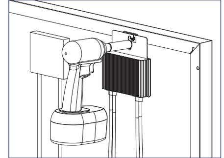
3) Tighten the mounting bolt on the MLPE Frame Attachment Kit to 12 lb-ft (144 lb-in).
